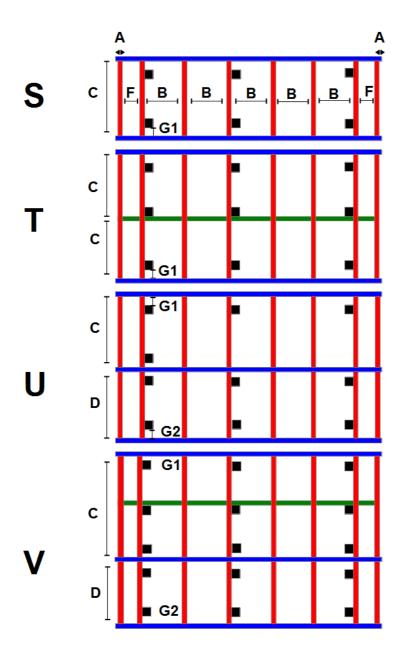
A= side recess 5/7cm 2/3", gap between joists B= approx 60/62cm 24/25" F = 39/41cm 15/16" C & D = support joist P = number of posts, G1 & G2 = the gap between front and back joists O/H is the approx. deck board overhang of the front and back joists
